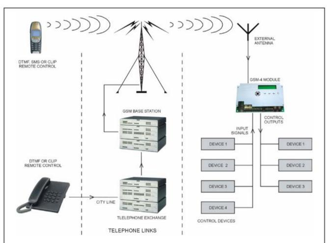
Figure 8. The ways of remotely controlling the status of outputs and the bypass of inputs of the module.
