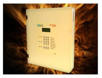
Microprocesor controlled panels 16 zones conventional fire alarm panel. 20 detector scan be connected to each zone and unlimited alarm buttons. The system checks the zones and sounder if they are close or open circuit than gives warning with flasher and sounder. Battery and energy interruption alarm. Can be program medeasly. Endoflineresistor LCD indicator. Alarm output with relay. Minimal dimensions Economi panels.
